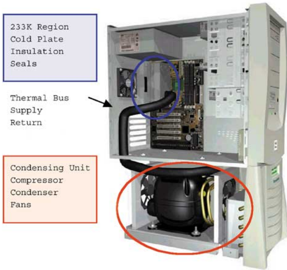
Figure20.7 Vapor compression cooling for Super G™ Computer
