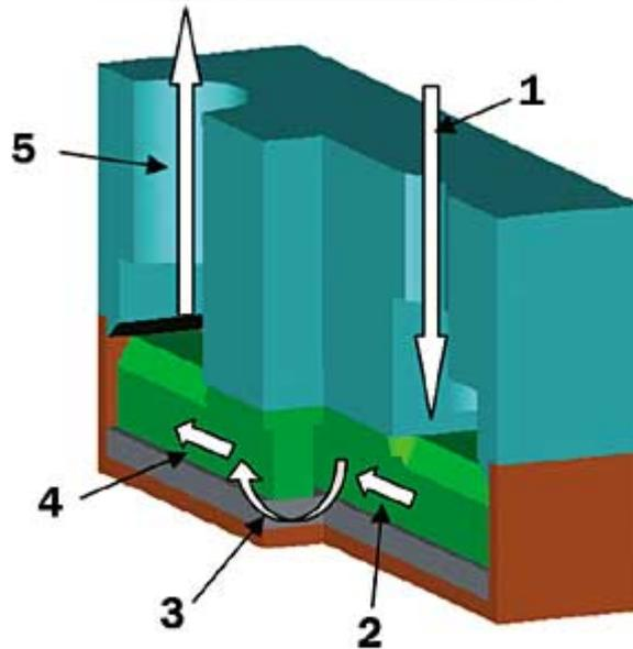
Figure 19.3b Coolant flow path
