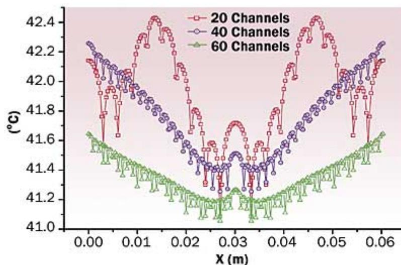
Figure 19.1b Temperature distribution at 1.0 m/s
