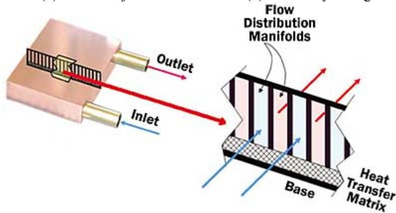
Figure 19.2 Normal flow cold plate (NCP) and manifold structure
