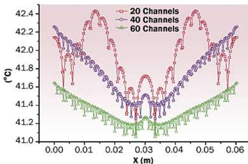
Figure 19.1b Temperature distribution at 1.0 m/s
