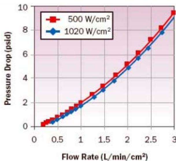
Figure 19.8b Ultra high flux NCP hydraulic performance
