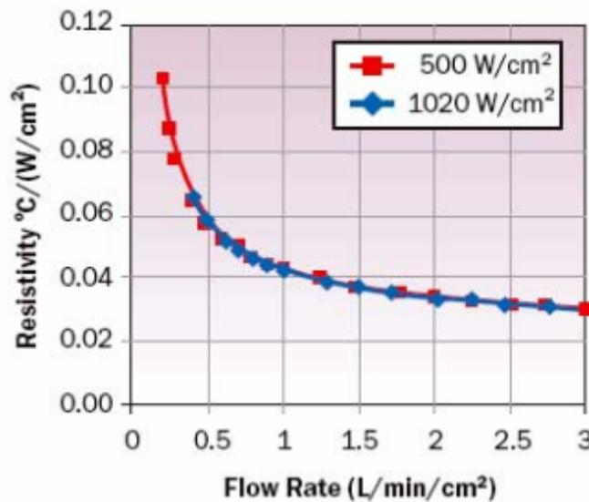
Figure 19.8a Ultra high flux NCP thermal performance
