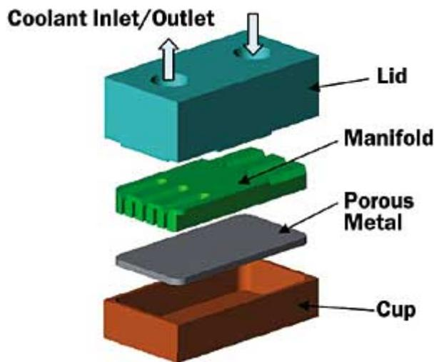
Figure 19.3a Powdered metal cold plate (PCMP) assembly
