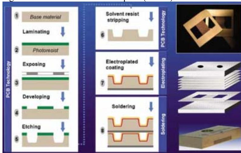
Figure 19.7 Microstructure cold plate fabrication process
