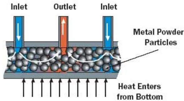
Figure 19.6 Powdered metal cold plate (PCMP) heat transfer matrix
