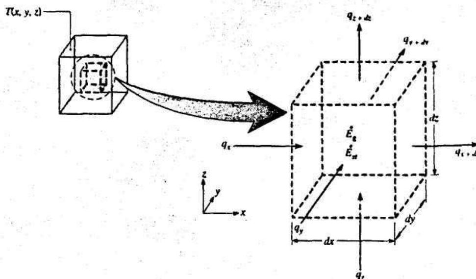
Figure 4.1 Differential control volume , dx dy dz, for conduction in cartesian coordinates.
