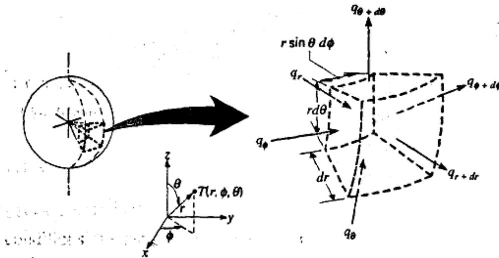
**Figure 4.3 Differential control volume , dr.r sin θ dφ .r dθ , for conduction analysis in spherical coordinates ( r,φ,θ)**
