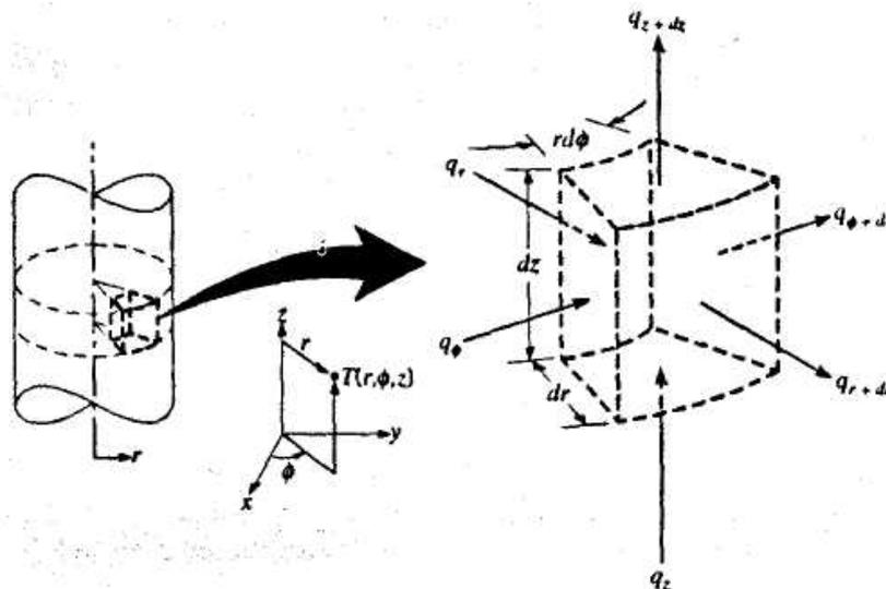
Figure 4.2 Differential control volume  $dr.rd\phi.dz$  for conduction analysis in cylindrical
