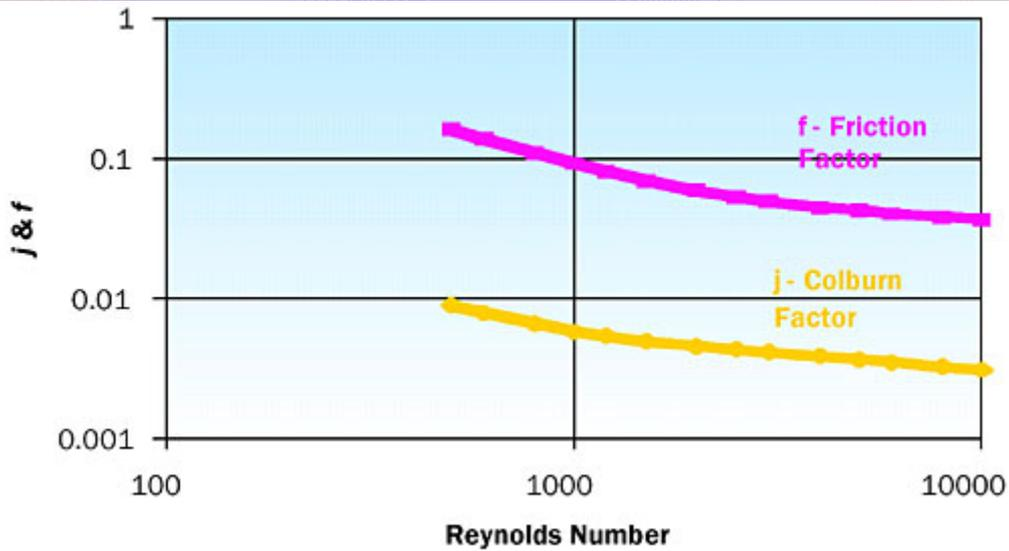
Figure 4.13 Finstock data # 14.77 from Kays & London (0.4 mm high, 0.15mm thick, 37.5 fins/mm, ST [0.330" high, 0.006" thick, 14.77 fpi, ST])
