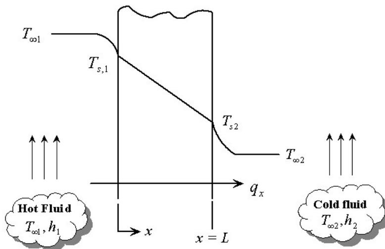
Figure 4.10 Heat transfer through a plane wall
