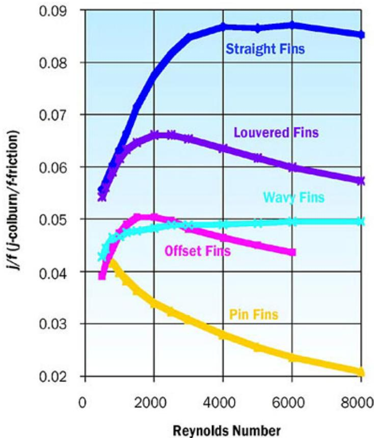
Figure 4.14 Heat transfer/pressure drop
