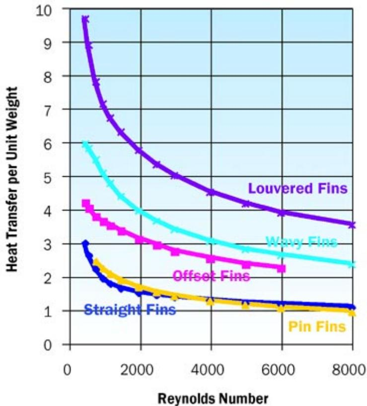
Figure 4.16 Weight figure of merit
